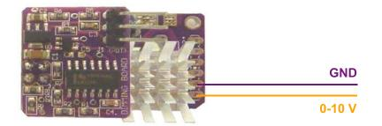
CONTROL SIGNAL: 0 V (LEDs OFF)
