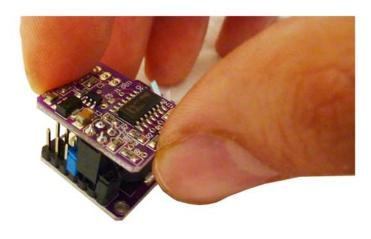
Black jumper must be in position 1 or removed.
